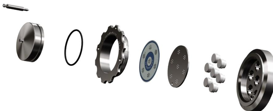
The Multi Micro Port 49 features 7 septa held in a housing and kept in place by an inner steel plate, which in turn is secured by a ring shaped nut.
